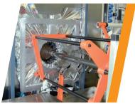
The egg and base are fed into the wrapping area, while a sheet pick-up system shapes the wrapping sheet in order to exert minimum pressure on the egg and minimise any risk of breakage. An adjustable contrast creates the necessary pressure on the sheet to control the wrapper adherence to the egg. When the sheet filling process is complete, the wrapping is tied with wedges arranged radially to close the sheet around the egg.
