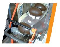
The machine's moving parts are entirely enclosed. The operator loads the egg manually on the feeder chain under completely safety. A loader automatically picks up the base and places it in the basket with the egg and together they are transferred to the packing area. At the same time, the reel unwinds the sheet according to the present length on the display, with either a continuous or centred print.
