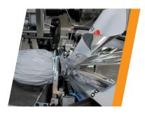
Once the egg is wrapped, it is transferred to the tying area and closed with a bowknot with a string in various diameters from 1.5 to 3 mm, unwound by a reel. A double bowknot is then made which makes it extremely easy to untie by simply pulling one of the ends of the string. The complete package is then placed on a conveyor belt to exit the machine and move to the packing area or another conveyor belt for the final packaging operations.
