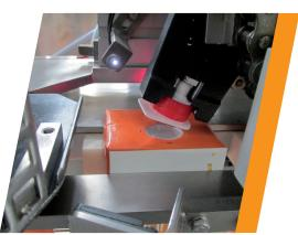
Possibility of applying clip caps as well as screw caps of different shapes and sizes on liquid packages (brick or gable-top) as well as on boxes for solid products.
