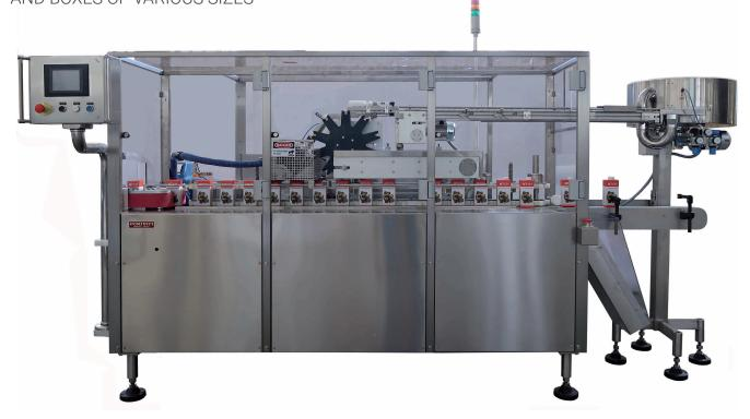
The caps are poured into a hopper in bulk, orientated and picked up continuously by the machine via suction cups. A hot-melt adhesive system allows an even layer of glue to be applied on the cap that is immediately applied with precision and pressed down on the package until it is perfectly bonded.
